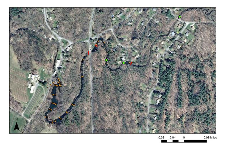
Figure 5. Map of bathymetric and depth of refusal survey data collected at Annandale Dam (orange points) and other inspection points (green). Locations of observed bedrock seams are shown as red lines. The furthest upstream bedrock seam shown on the map corresponds with the upstream extent of the impounded water surface during low-flow conditions.
