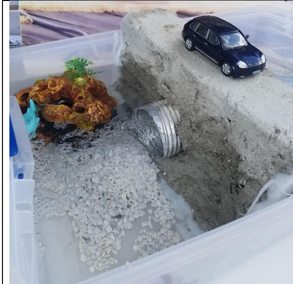
Figure 36: Demo of good culvert design. Culvert is below stream water level.
