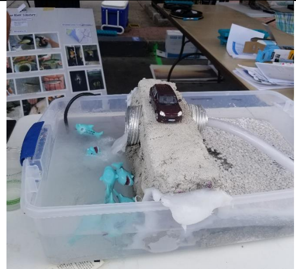
Figure37: Demo of bad culvert design. Culvert is above water level. Fish can't swim up waterfall. (Ice chest in back stored 40+ ice trays filled with Sing Sing Kill water ice cubes for aquarium).
