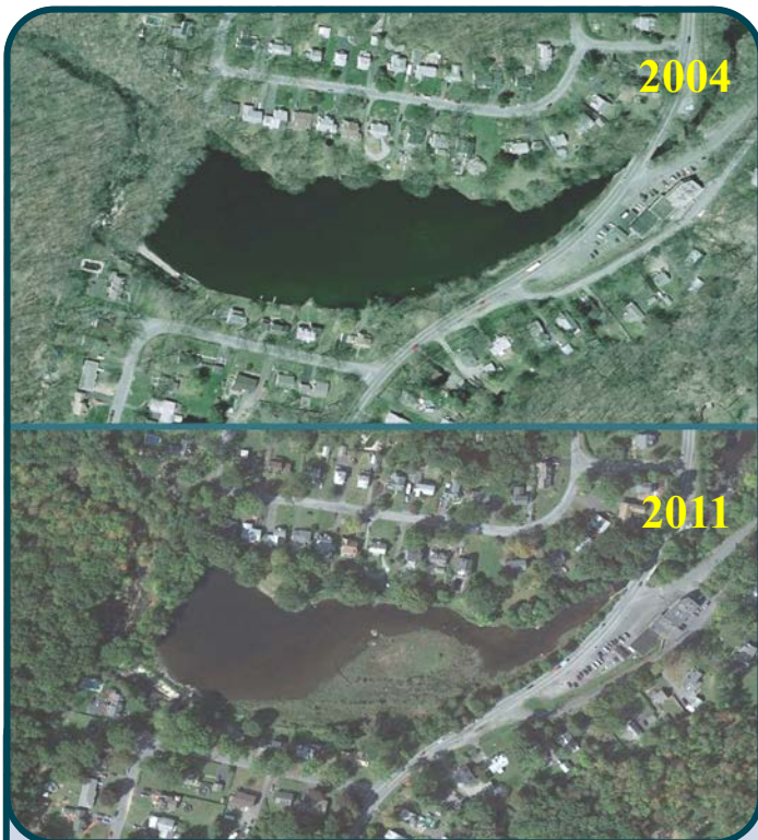
Figure 2: Winona Lake in 2004, prior to 2007 breaching of dam's spillway, and in 2011. Images courtesy of Google Earth.
