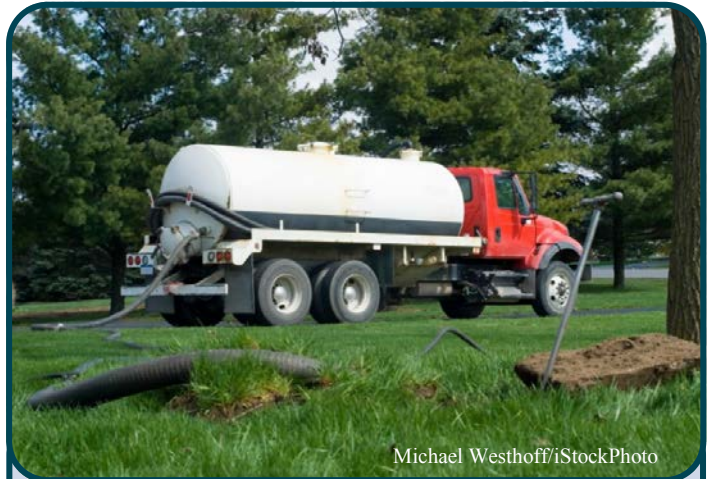
Photo 2: Periodic pump outs are required to ensure systems function properly.
